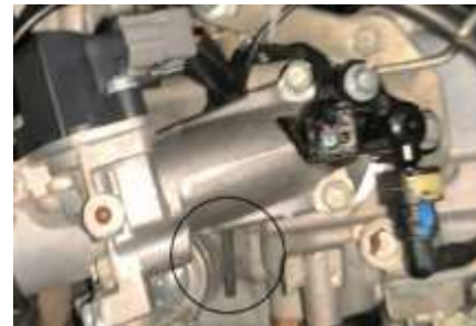
Figure 3. Placement of DS18B20 Temperature Sensor on Motorcycle Engine Block.
