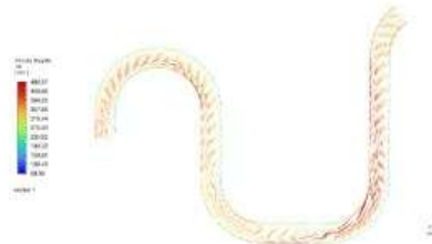
Figure 9. Velocity Vector of Gas Flow Magnitude at Variation B
