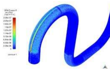
Figure 15. Contour of maximum erosion rate on manifold pipe
