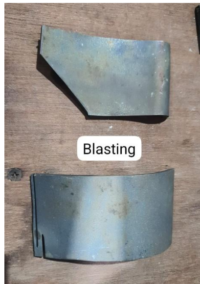
Figure 14. INCONEL 939 specimen after the heat-in process Source: Authors' experimental data (2025)
