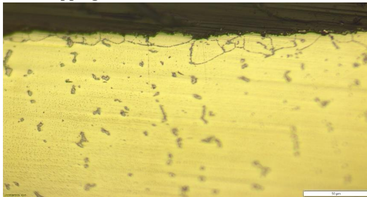
Figure 10. Cross Section Cross-Section in INCONEL 939 after soaking with HCl 12 Mol for 10 hours
