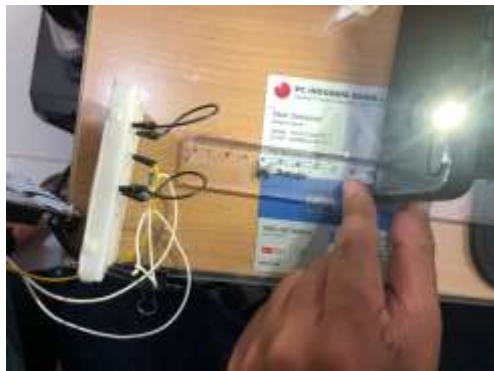
Figure 3.3 LDR testing with HP flashlight light LDR Sensor 1
