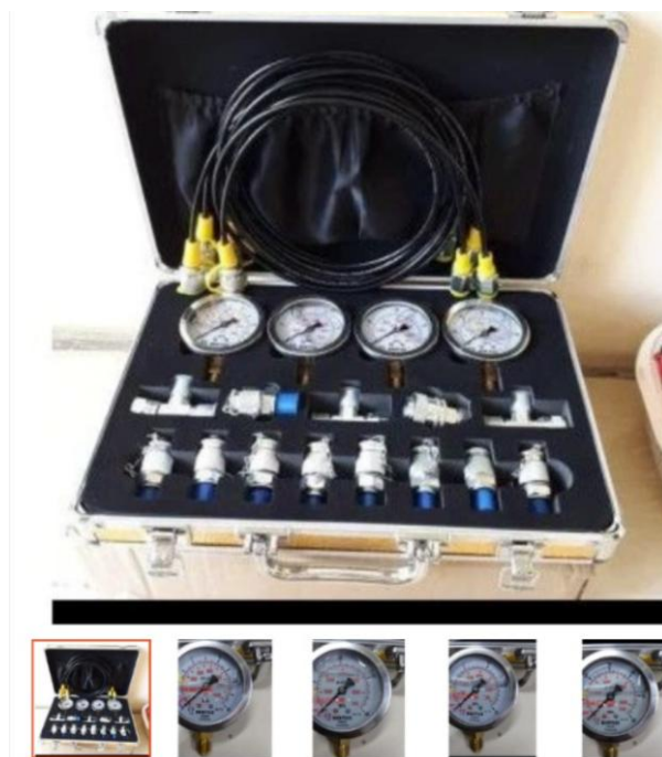
Figure 4. Genuine Komatsu pressure gauge tool set (four gauges and coupler connectors) already available internally in the Plant Department.
