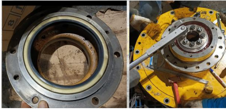
Figure 2. Propulsion/drive motor component removed from the unit due to damage suspected to be related to the hydraulic PPM not running optimally
