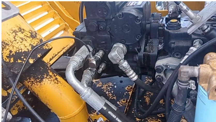
Figure 5. Genuine Komatsu PPM coupler (part number 799-101-5230) after installation on the PPM port of the Sakai compactor unit
