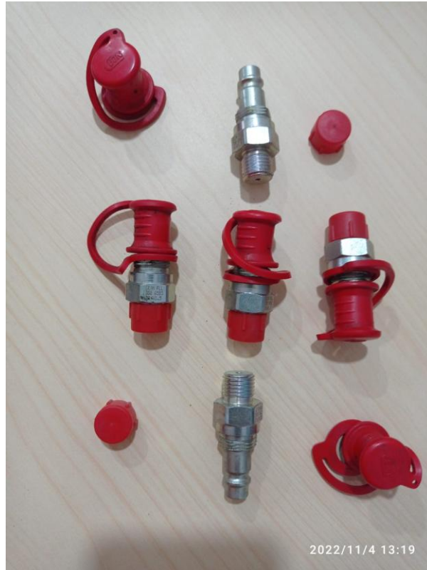
Figure 3. The original Sakai manufacturer PPM coupler (left) and its incompatible connection with the Genuine Komatsu pressure gauge tools, before modification.
